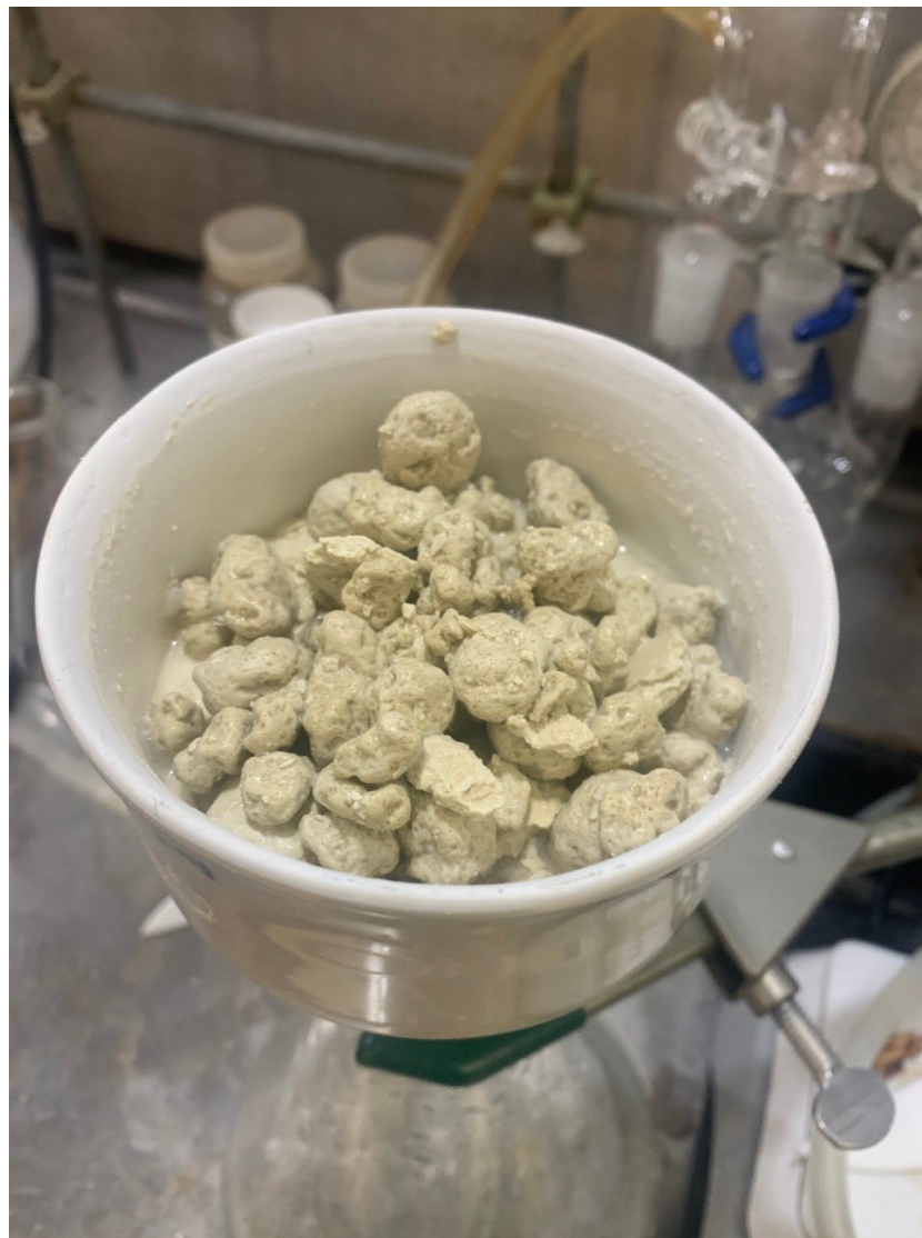
Figure 4. Photograph of polyureas obtained from stirring of 50 g/L pMDI in distilled water for 14 d:
